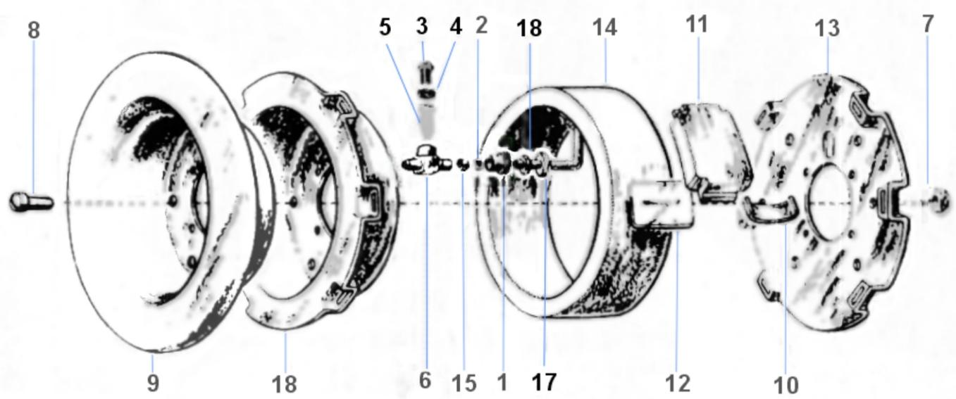
Brake Assembly: Part Nbr: D2-113
